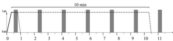
**Fig. 2.** The time course of the sham and verum stimulation. Both conditions began with a 20 s fade-in phase; in the case of sham stimulation the current was ramped down in 10 s after 30 s of stimulation, in the verum case the stimulation lasted for 10 min, after which it was ramped down in 10 s. During the course of the session the participant was prompted to report the cutaneous perception (grey bars).
